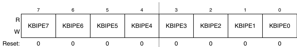
Figure 9-4. KBI Pin Enable Register
